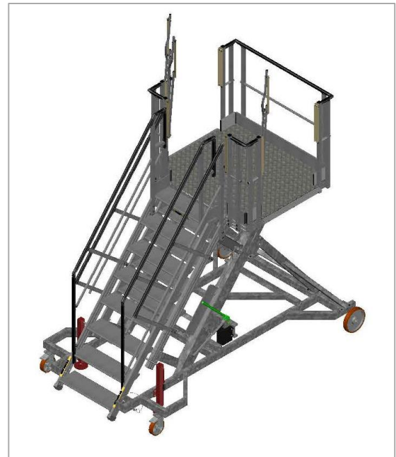
3D view stepladder in low position with safety gates (guillotine type) lifting (mounting and lateral sides)
