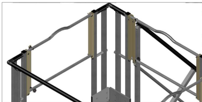
3D view stepladder safety gates (guillotine type) in close position.
