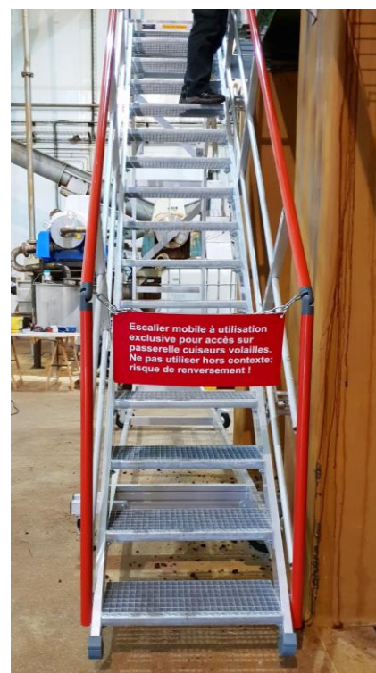
Mobile access staircase – useful width 600 mm – grating steps depth 280 mm – 4 swivel wheels with brakes for easy moving. This staircase is regularly moving to allowed crossing truck.
