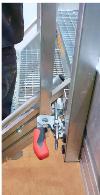
Access staircase fixing on platform by « hopper » system
