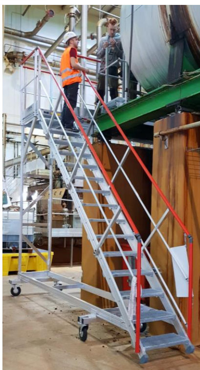
Mobile access staircase – useful width 600 mm – grating steps depth 280 mm – 4 swivel wheels with brakes for easy moving. This staircase is regularly moving to allowed crossing truck.
