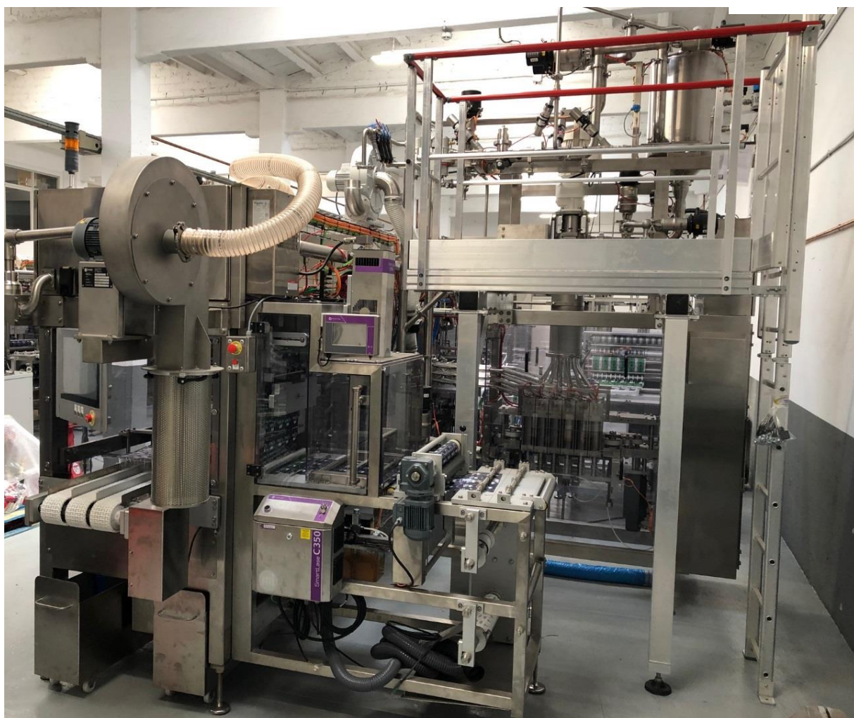
Aluminum platform on yoghurt packaging line. Capacity of load: 200 kg/m 2
