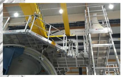
Fixation system of tower access to hub – platform standd on its foot – galvanised steel bracket screw on the hub for receive the gangway.
