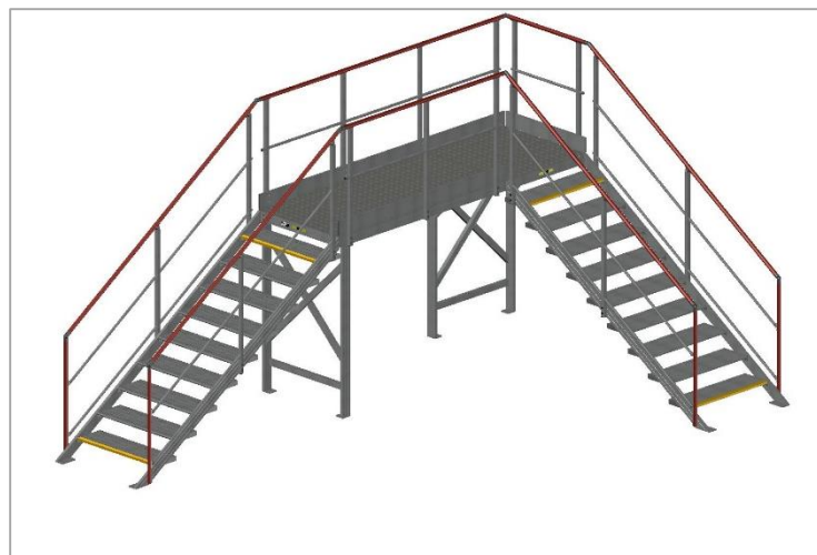
Double access staircase 3D view
