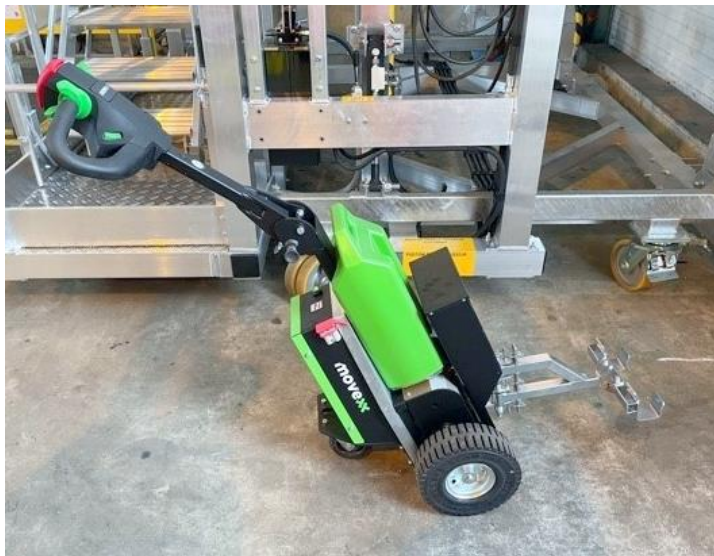
Option: electric pusher with 3 gripping points, visualized by yellow sticker (1 on the front, 2 on lateral) for easy movement at 5 km/h maximum.
