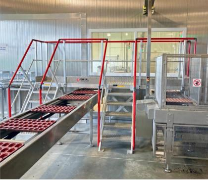
Raw extruded aluminum gangway 100x30 mm for « before demolding » station crossing
