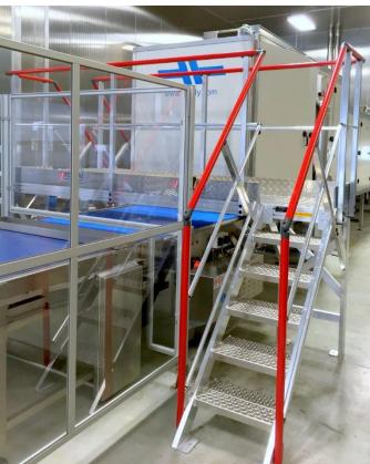
Raw extruded aluminum gangway 100x30 mm for « after demolding » station crossing
