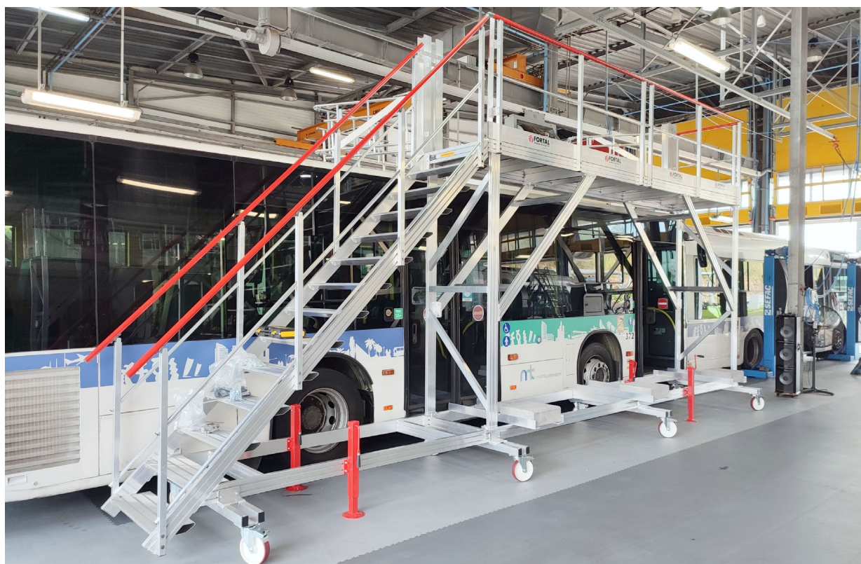
3D view mobile platform with articulated guardrail deployed
