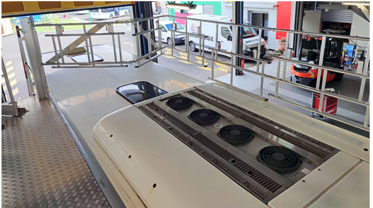
3D view mobile platform with articulated guardrail fold
