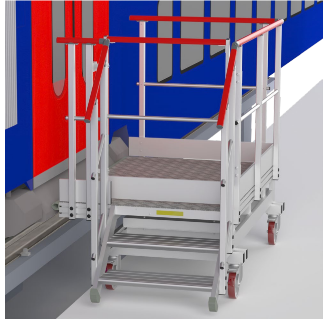
3D view mobile platform for door access
