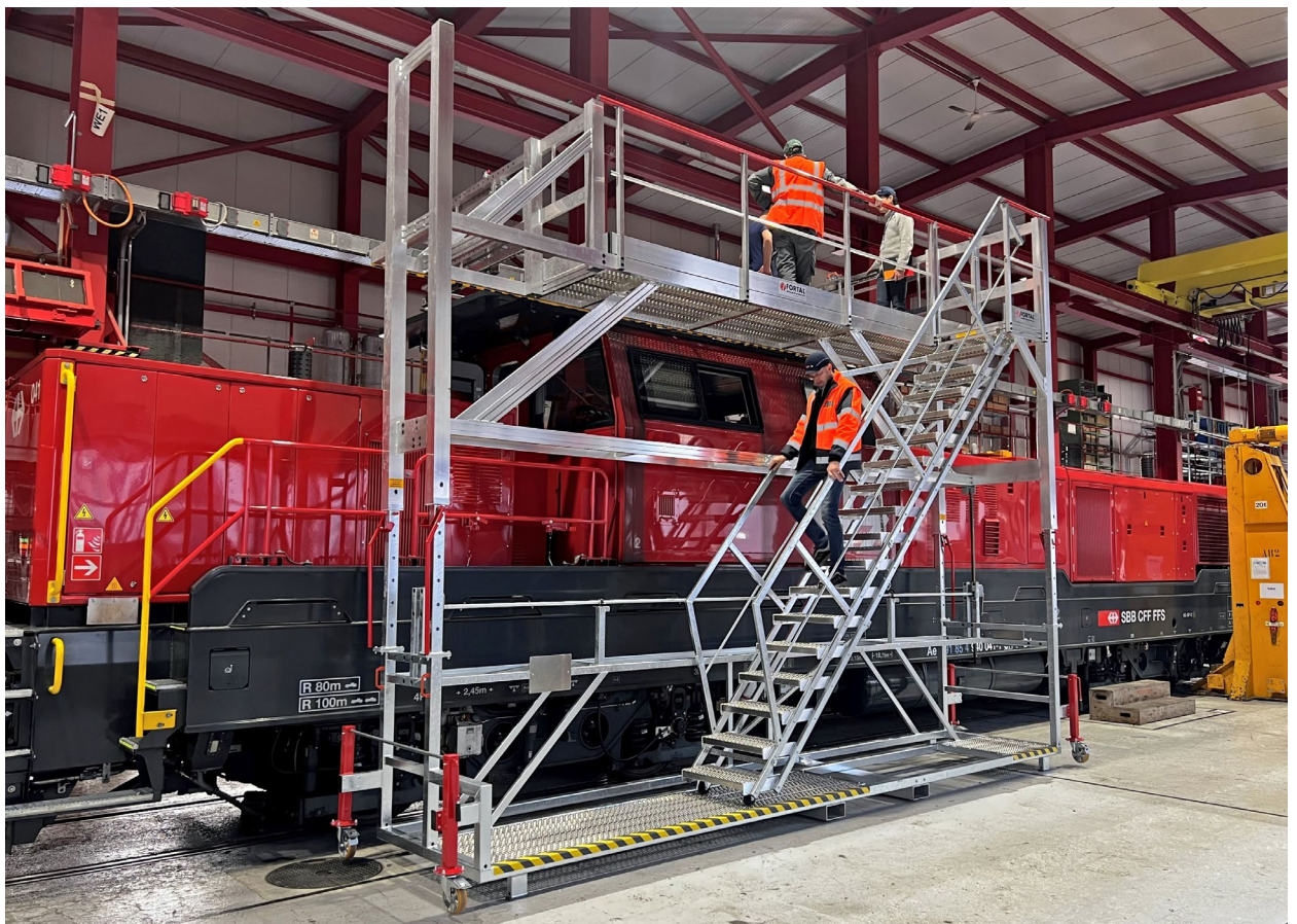
3D view articulated guardrail deployed on the train roof
