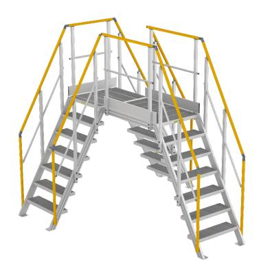
**Triple-access walkway designed to provide safe crossing over a conveyor** within a winery. Constructed entirely from extruded aluminum, it offers ergonomic access from three sides and withstands the humid conditions typical of viticultural environments. Its design, featuring integrated guardrails and a non-slip structure, ensures safe, long-lasting use adapted to production demands.
